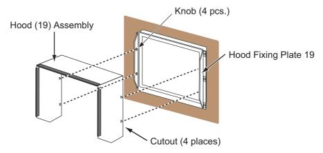
8. Press the top of the hood (19) assembly to set the knobs in the cutouts.
